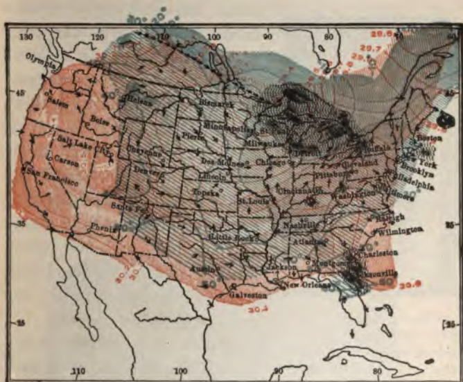
FIG. 116. One of the Washington weather-maps. The red lines join places where the barometer is the same. The blue lines join places where the thermometer is the same.
